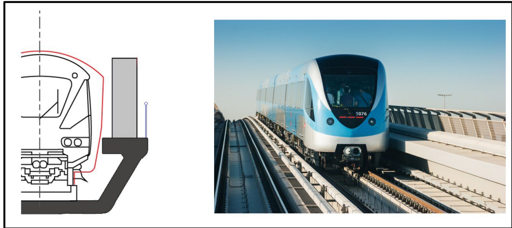
4-13. Cross-Section of U-Girder Showing Top of Parapet at Required Evacuation Path Height (Photo Courtesy of SYSTRA IBT)
