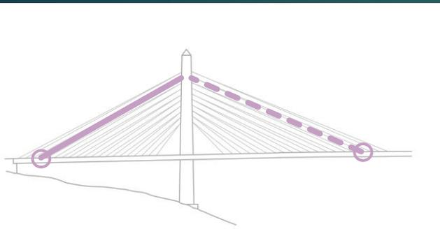
Stay 17 Back and Main Span - Carbon Fiber Strand Forces
