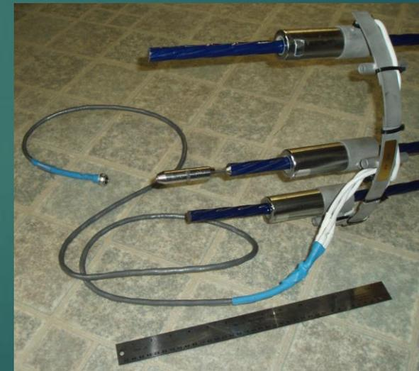
DSI-DYNA Force™ monitoring system for steel stay strands (at each anchorage)
