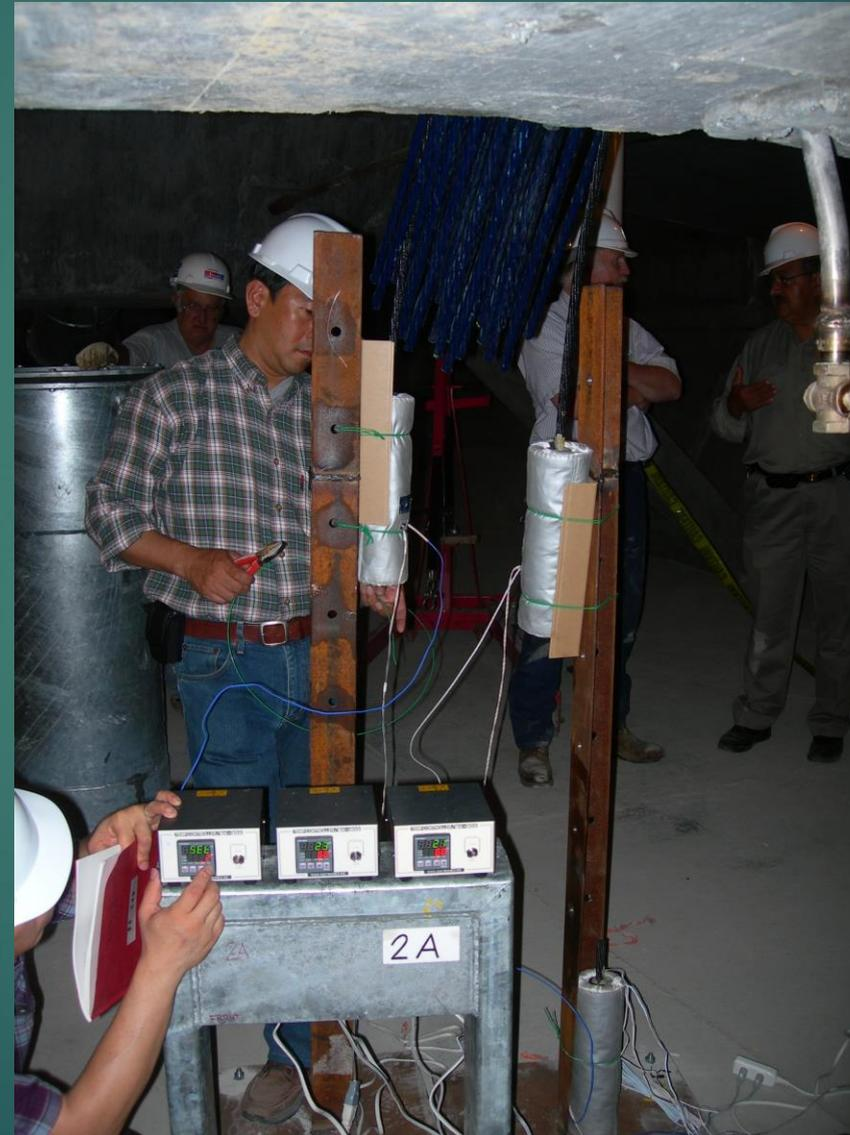
Temperature monitoring of HEM during curing
