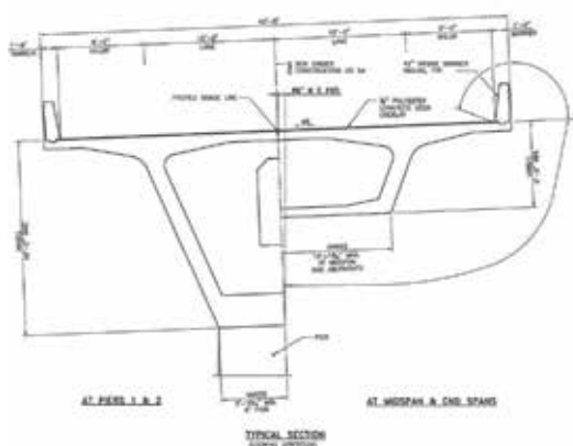
Typical bridge section showing the box-girder depths, which vary from 18 ft at the piers to 8 ft at midspan and at the abutments. Figure: New Mexico Department of Transportation.
